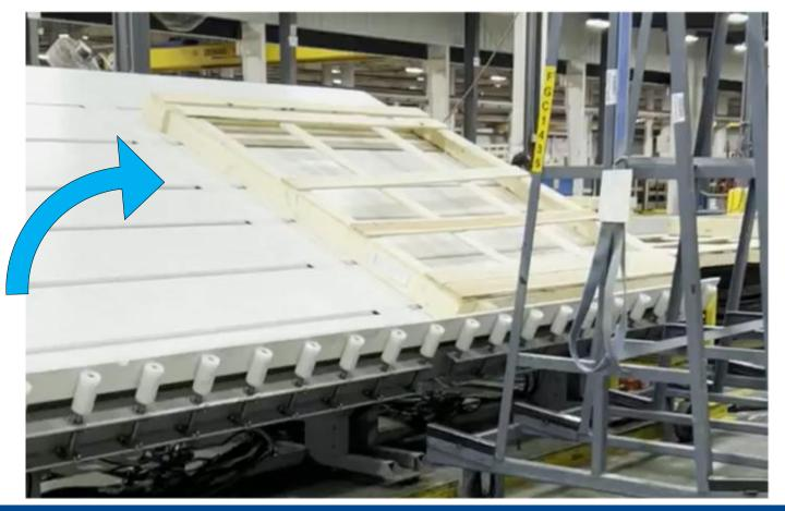
Box is Pushed from Tilt Table to Cart Using Push Pistons assembly
